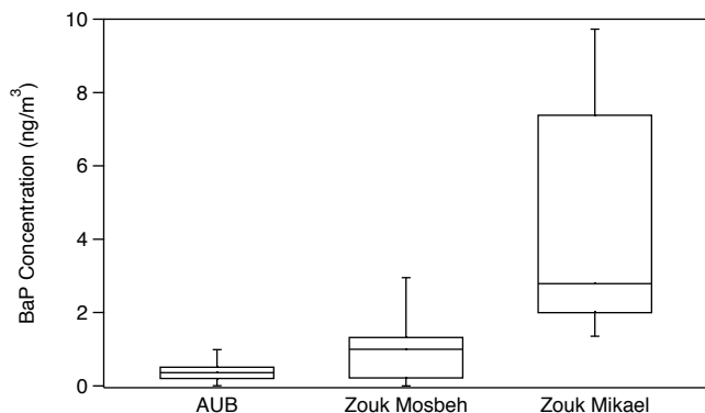
Figure 4-4 Box Plots of BaP Concentrations Measured at AUB, Zouk Mosbeh and Zouk Mikael. Whisker Bottom, Box Bottom, Box Top and Whisker Top Represent 10, 25, 75 and 100 Concentration Percentiles Source: Baalbaki et al., 2018
